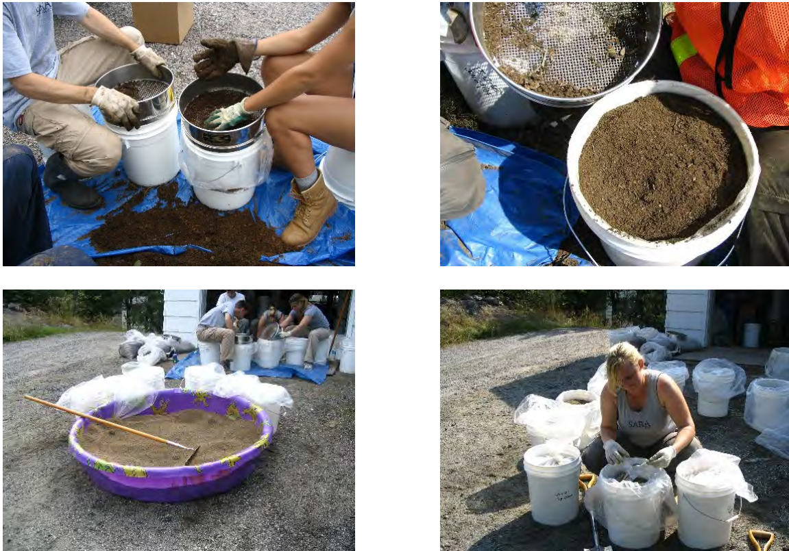
Figure 3-7 Preparation of Homogenized Soil Samples: a) & b) Sieving Bulk Samples; c) Mixing to obtain a Homogenized Sample; and, d) Collecting a Representative 400 g Sample and Packing Homogenized Soil Samples.
